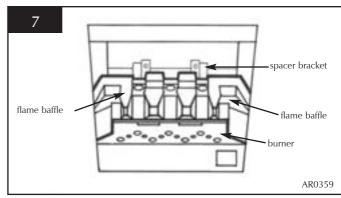
• Put the flame baffle onto the burner and push against the rear tray lip, Diagram 7
